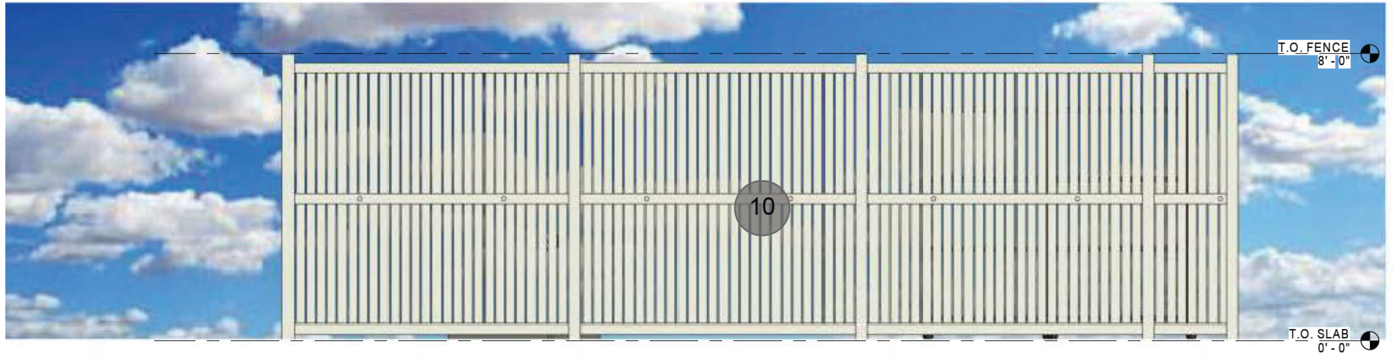
④ TRASH COMPOUND - REAR ELEVATION 3/8" = 1'-0"
