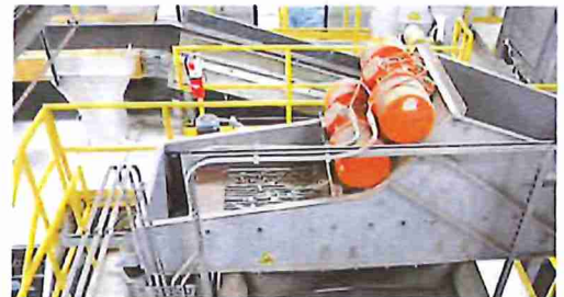
4: A series of screens are used to extract other contaminants.
