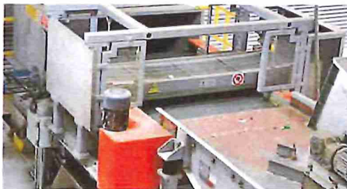
3: A magnet and eddy current are used to extract steel and aluminum which will be recycled.
