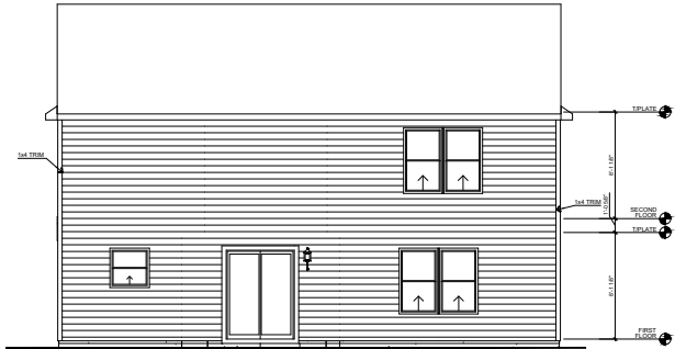
REAR ELEVATION - SLAB
