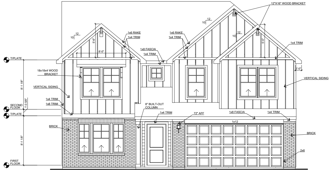
FRONT ELEVATION E - SLAB - BRICKFRONT C
